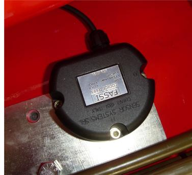
**Digital tilting sensor** with a double axis XY mounted on the crossbeam of the crane base.
