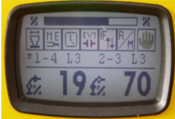
The display of the user's panel shows that the crane is working in the working zone **1-4** prearranged for the **level L3** and that the zone **2-3** is also prearranged to work in **level L3**. This means that the supports for the lateral extension of the outriggers are completely extended on both sides or at least they overcome the middle.
